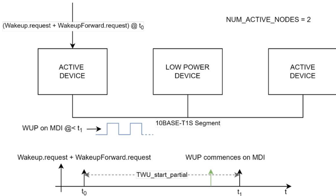
Figure 7-3--TWU\_Start\_partial diagram
