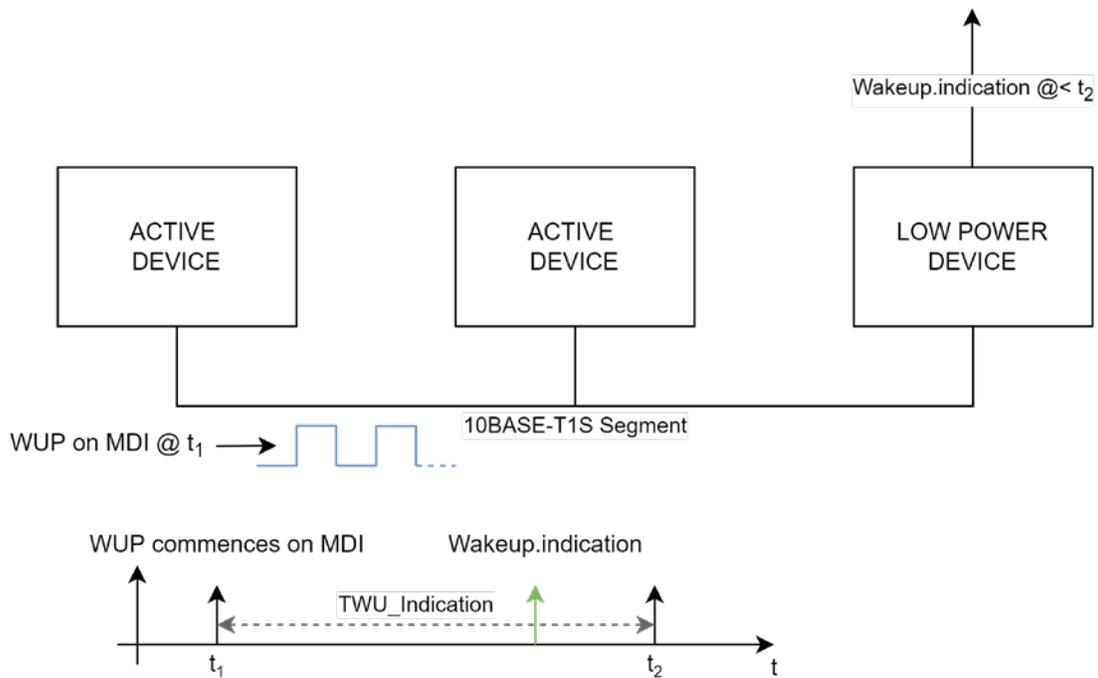
Figure 7-4--TWU\_Indication diagram
