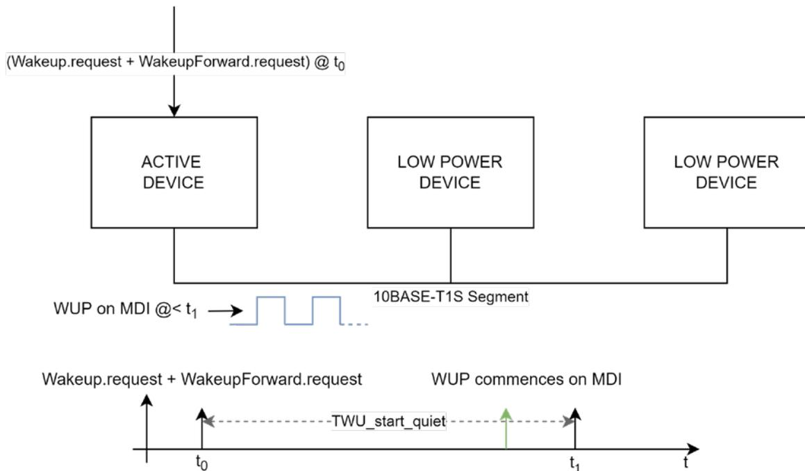
Figure 7-2--TWU\_Start\_quiet diagram
