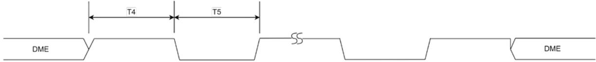
Figure 147-14--WUT encoding
